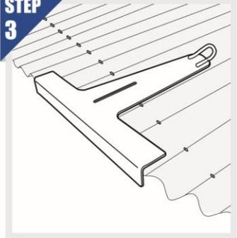
SIT THE ANCHOR ON TOP CORRUGATION OF ROOFING IRON AS SHOWN
